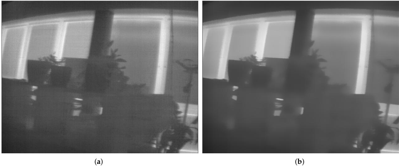
**Figure 1.** Example of bilateral filtering applied to a thermal camera image demonstrating noise reduction while preserving edge details. Areas with no visible edges are smoothed, while edges remain sharp. (a) Before denoising. (b) After denoising.
