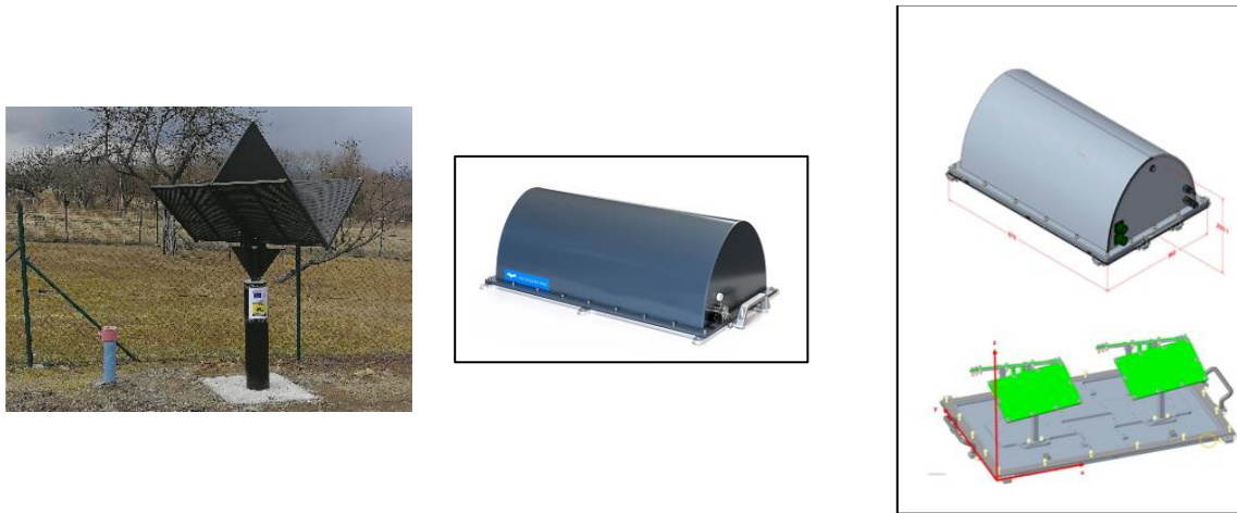
FIGURE 8: PASSIVE CORNER REFLECTOR (LEFT) AND COMPACT ACTIVE TRANSPONDERS (MIDDLE, RIGHT)
