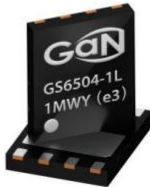
FIGURE 4: GaN SYSTEMS GS-065-004-1-L HEMT THAT IS SELECTED AS THE DUT
